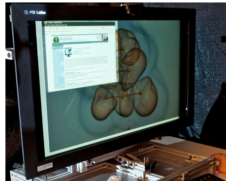
Figure 7. Example of a 2D web browser running alongside the 3D autostereo Nanovolt application.
