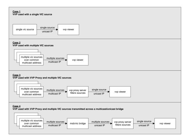
In this case VVP does not need to perform filtering of UDP packets to find a specific source. VVP must be configured with the IP address and port number that the VIC source is using to transmit video. The VIC source will not receive reports from VVP.
