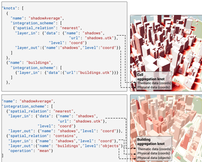
Fig. 4: UTK abstracts spatial joins through the use of knots. Top: Knot integrating thematic and physical layers. Bottom: Knot integrating a thematic layer with the average per building.
