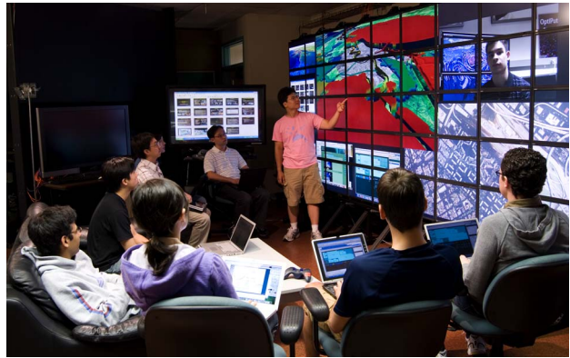
Fig. 4. The LambdaVision—a 100-Mpixel LCD OptIPortal was built from 55 20-in LCD panels and driven by a cluster of 30 computers (2005).
