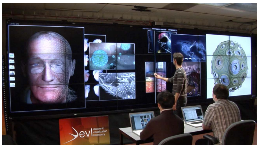
Fig. 6. A user partitions on the work space in SAGE by drawing wall dividers with his finger.
