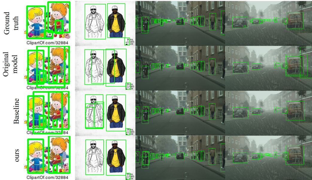
Figure 8. Qualitative results of fully test-time adaptation for object detection. The first row is the ground truth of each image, the second row is the results of the pre-trained detector, the third row is the results of the self-training baseline, and the last row is the results of our proposed method. The object detection results are localized as green boxes.
