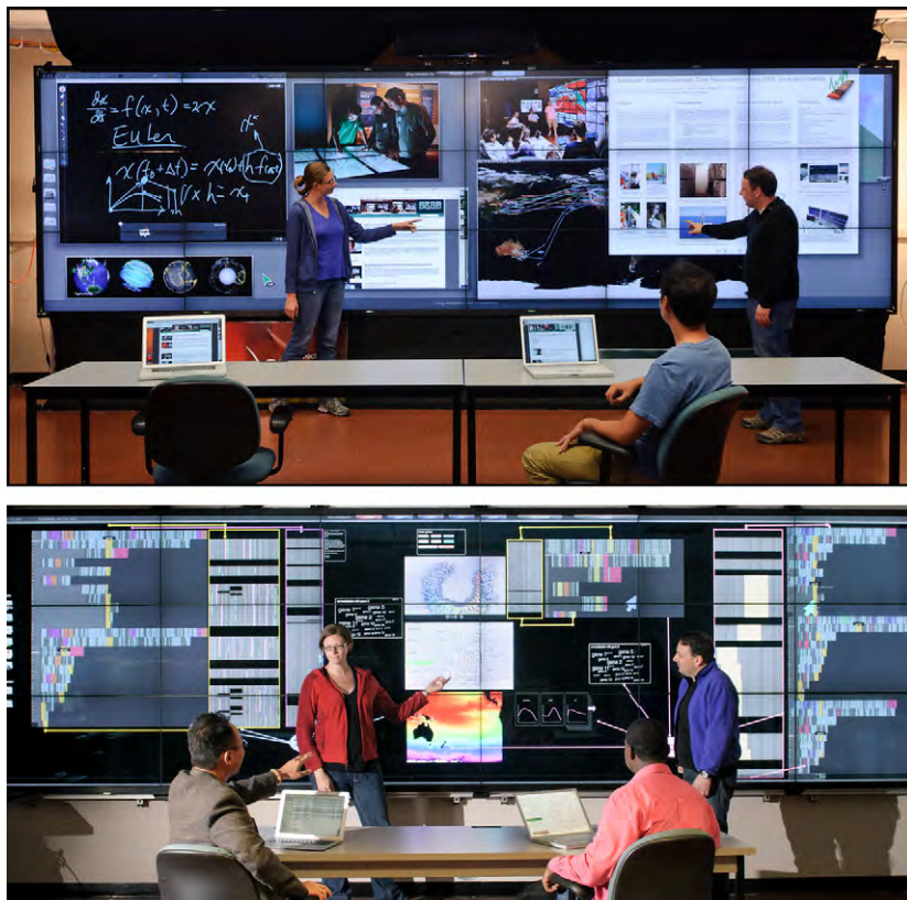
Fig. 1. A single machine-driven tiled-display wall running SAGE at the Electronic Visualization Laboratory in the University of Illinois at Chicago. The 20' by 6' display wall is made up of 18 LCD panels with a total resolution approximately 17 megapixels.
