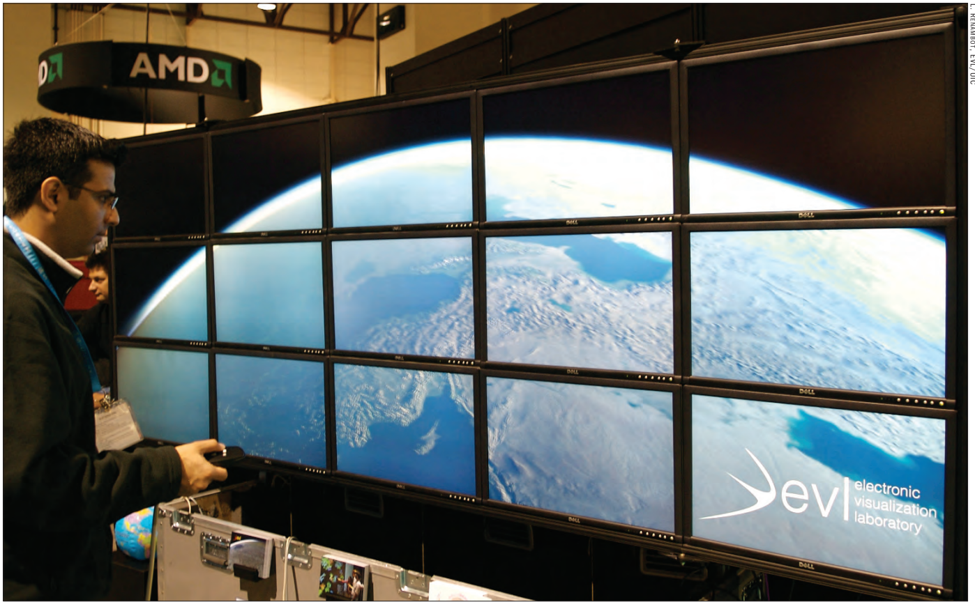
Figure 2. Tellurion, a real-time planetary-scale data visualization being developed by EVL/UIC Ph.D. candidate Robert Kooima, is shown here on the Calit2 OptiPortable (the portable OptiPortal) at SC07. Tellurion uses NASA's Blue Marble Next Generation and Shuttle Radar Topography Mission data.
